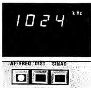
Front-panel section: right-hand display/keyboard for modulation frequency and distortion measurements
